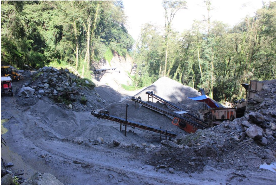
Figure 7-10:Crusher setup and aggregate production
